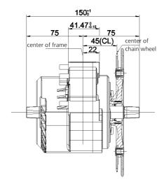
Chain line(CL): 45/48mm Shaft standard: JIS
