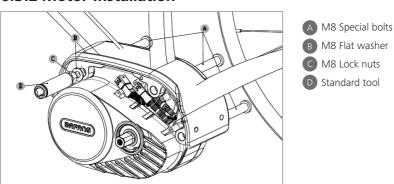
1) Align the three mounting holes in the drive unit, with the mounting holes in the bike frame. From the right side of the bike frame, insert three special M8 bolts through the frame and motor to keep the motor in place.
